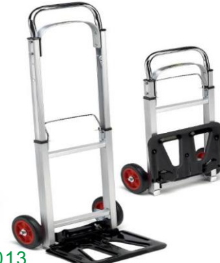
KH013 Product size: 420x400x1080mm, Folded size: 190x400x710mm, Max capa:90kg, Alu platform: 240x355mm Rubber wheel: Φ150mm,
