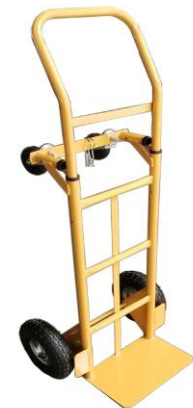
KH047 Product size : 1400x500x420mm Max capa : 200kg Steel frame,powder coated finish Wheel: 10"x3.50-4 4" castor
